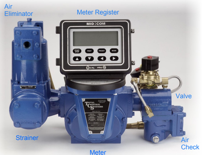
Series 700 petroleum meter shown, with electronic registration and solenoid-operated control valve.
